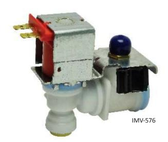
The Robertshaw<sup>®</sup> S-86 single and N-86 dual Water Valve Series are automatic icemaker valves for residential refrigerator icemakers. The N-86 valve allows individual control of water flow through two outlets by using a single inlet for water to the door and for water to fill the icemaker.
